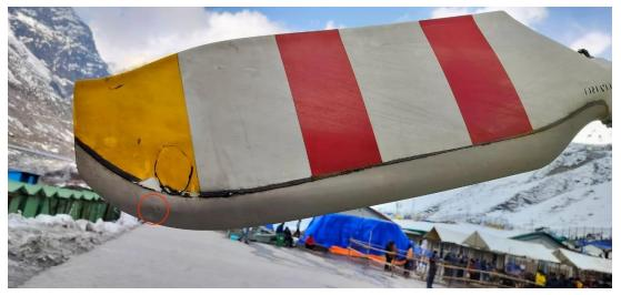
Figure 2: Small dent on tail rotor blade
